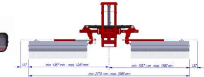
3966 mm 2775 mm 760 mm 975 mm Hydraulic 200 mm Hydraulic ( 2 x 500 mm) 1000 mm (2000 mm without Shields) 2-4 bar Up to 10 km/h Up to 1-2 ha/h Custimized bracket 135 Kg
