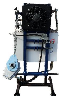
Hydraulic pump+ 75 Lt oil tank + Cooling Radiator
