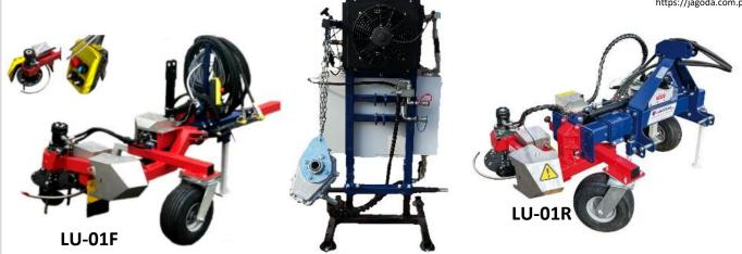
Hydraulic pump+ 75 lt oil tank + Cooling Radiator
